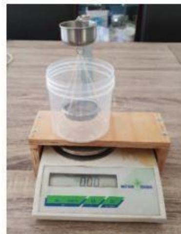
Figure 2. SG setup on the scales with a suitable water container. No part of the basket should touch the sides or bottom of the container.
